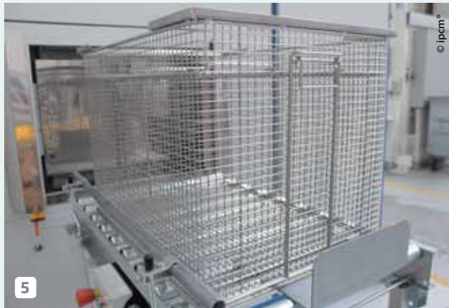
5 A special feature of the Ilsa machines is that the basket containing the parts can be designed according to the client's washing requirements.
