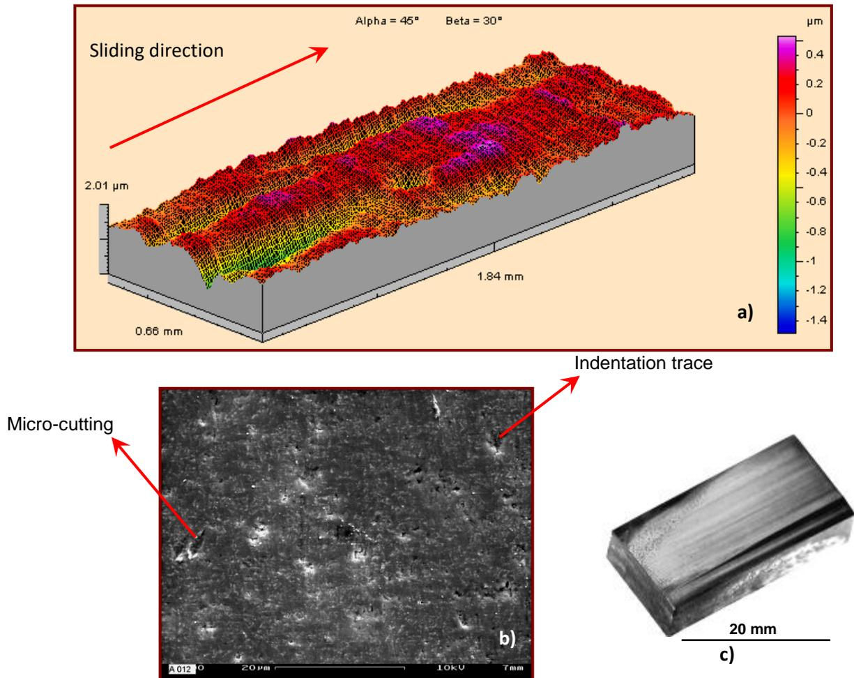
Figure 3: a) Worn surface morphology of thermally sprayed  $\text{Cr}_3\text{C}_2\text{-NiCr}$  coating caused by slurry abrasive measured by white-light profilometer (Altisurf 500-Cotec), b) SEM micrograph of the worn surface, c) macrograph of the worn testing sample.
