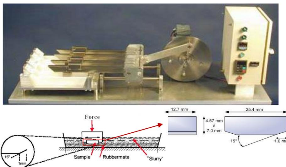
Figure 1: Slurry abrasion test built-up with the testing sample geometry
