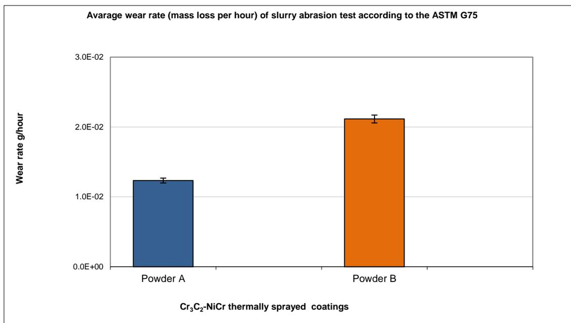
Figure 2: Wear rate of test samples subjected to slurry abrasion ASTM G75, for 6 hours with two hours of intervals.
